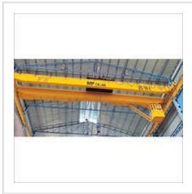
25T-10T Double Girder Crane
